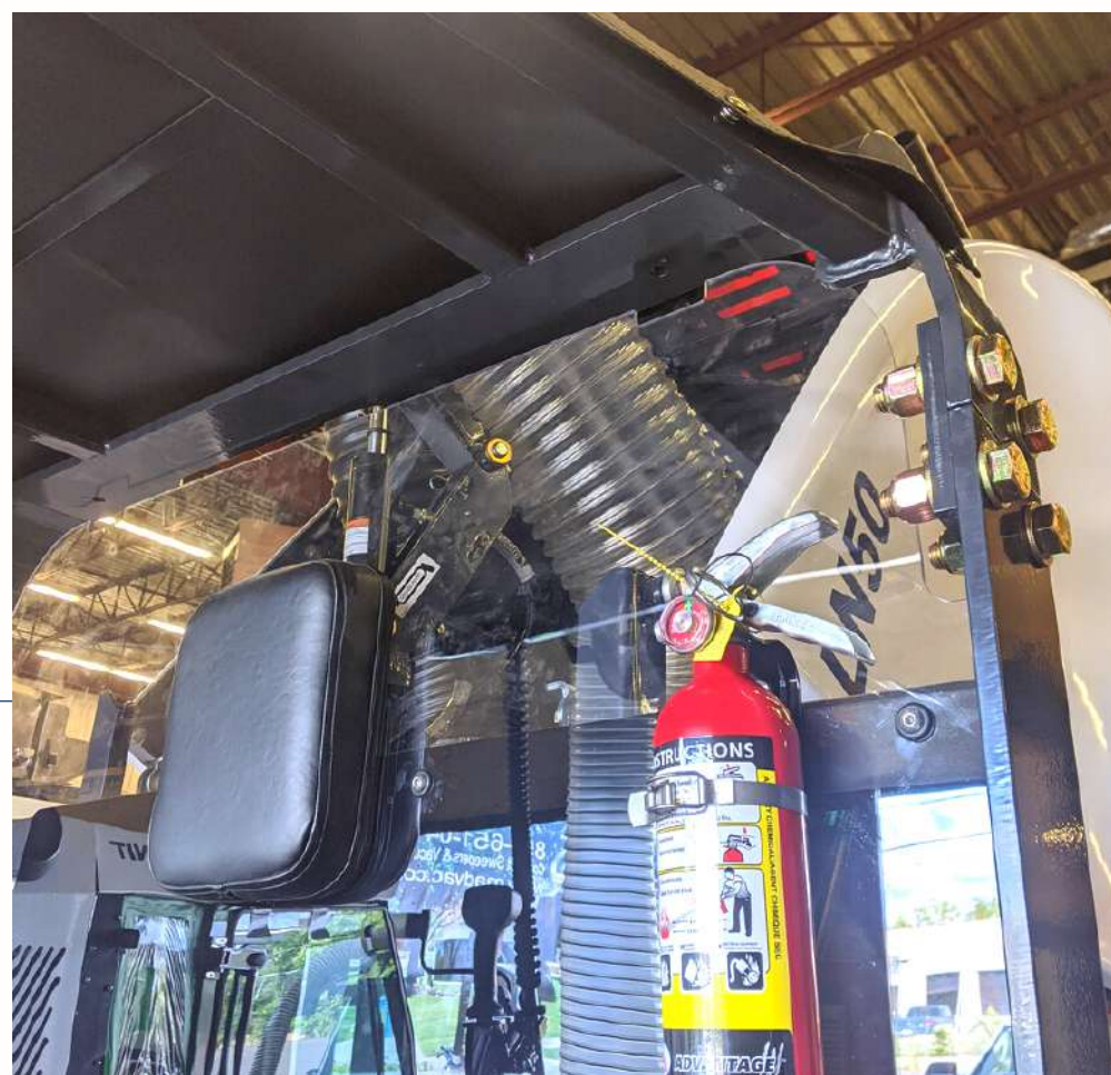
R.O.P.S. rollover protection system
