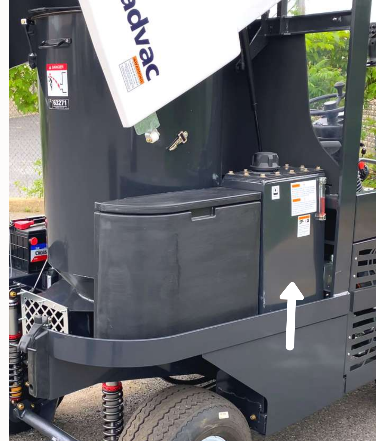
Hydraulic tank with 12.5 gal. (48 L) capacity for both the traction and the vacuum systems
