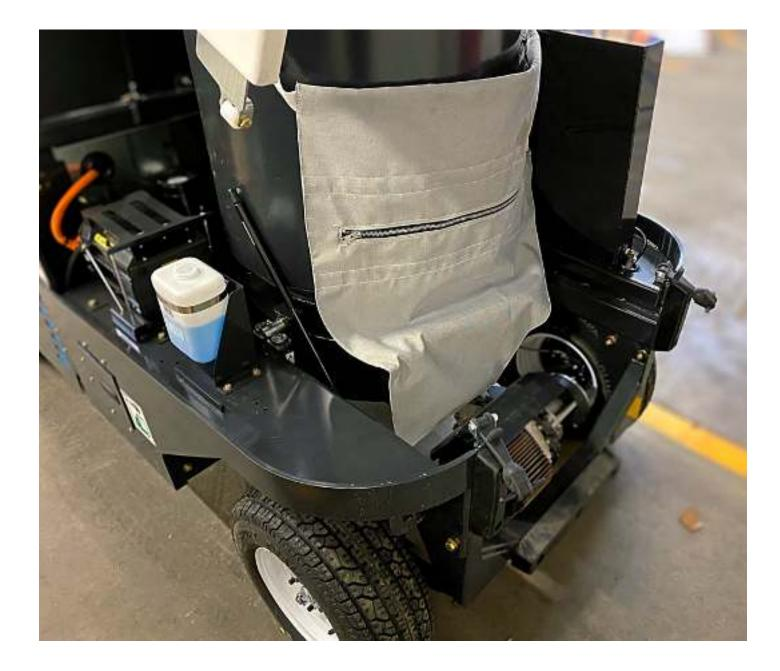
Exhaust bag reduces dust particles that can escape from minute holes of special Madvac collector bags (or Kevlar bin)
