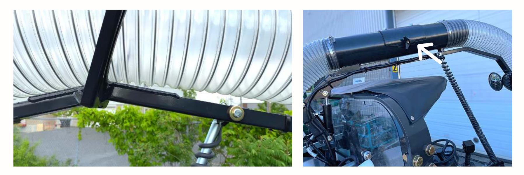
For operator safety and easy displacement of the boom | removable plate to access top hose
