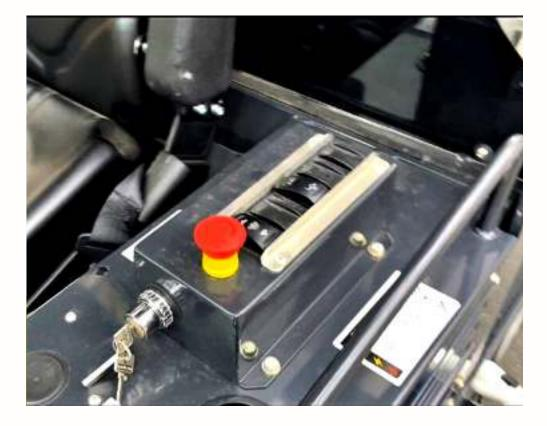
Console accessory box with USB / 12V aux outlet and rocker switch for optional water mist system and 48" wide vacuum head
