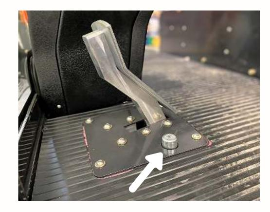
Foot step helps operator climb on board easily and safely Foot activated horn gives operator more ease and convenience than pressing the turn signal lever
