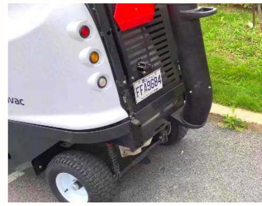
Optional -tire flat proofing (liquid sealant) License plate holder
