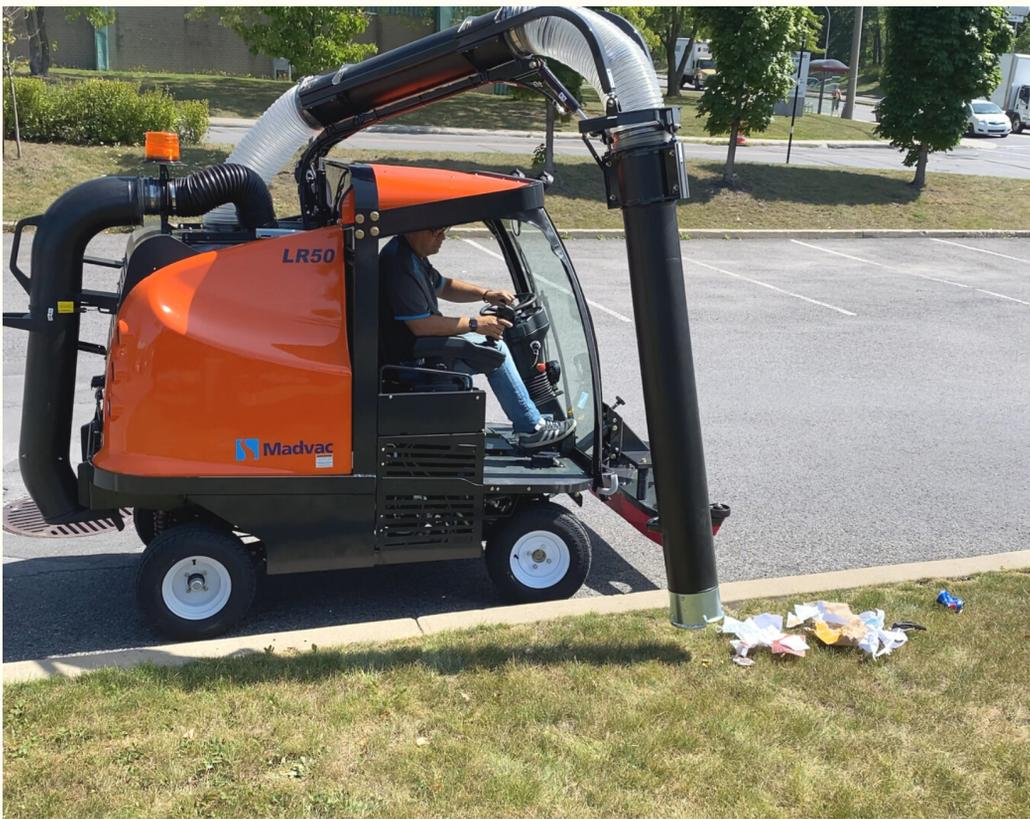
Ergonomic 6-position robotic joystick allows effortless displacement of the boom
