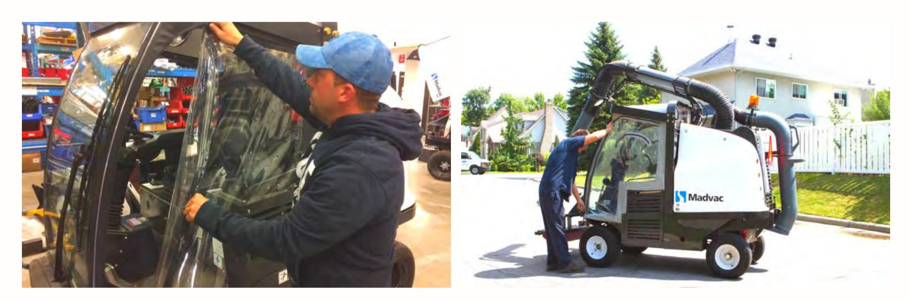
Enclosed cab with either heated or non-heated windshield, and vinyl doors
