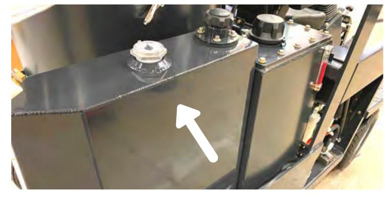
Optional – intermittent water mist system with 10.17 gal. (38.5 L) water tank: controls dust and reduces risk of cigarette butt fire inside the container
