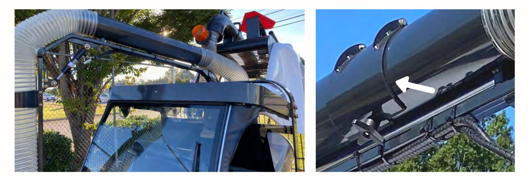
For operator safety and easy displacement of the boom | removable plate to access top hose
